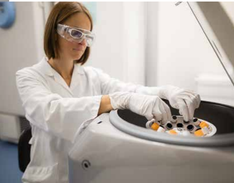
Centrifugation of blood samples in preparation for serological testing
